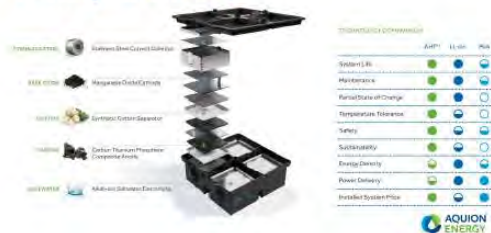
Figure 33: The energy storage system explained, courtesy of Tom Griffiths, SPECIFIC
